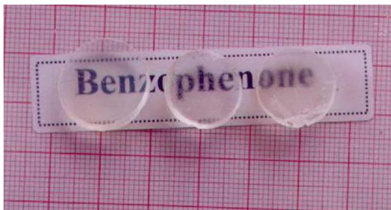
**Figure 9.** Cut and polished samples from USC grown crystal.
