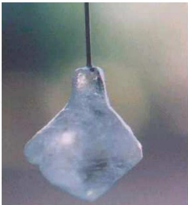
**Figure 6.** Grown crystal with high shoulder angle.
