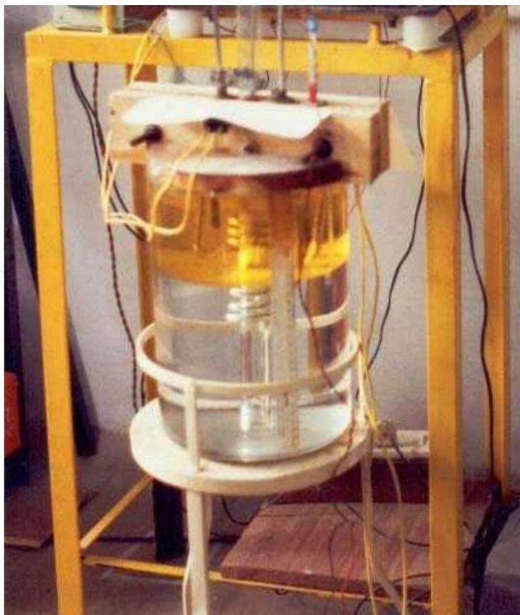
**Figure 1.** Transparent vertical Bridgman growth system.
