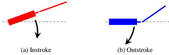
Fig. 6. Definitions of the half-cycle stages in yawing movement
