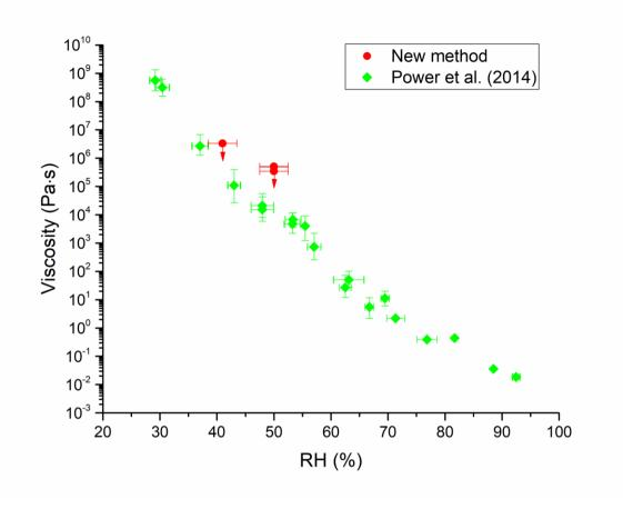
Figure S4. Viscosity as a function of RH for sucrose-water particles. Red dots represe
