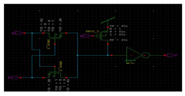
Figure 6: Proposed Nano-Wire based XOR gate
