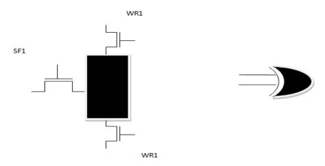
Figure 3: Nano wire based XOR Gate and Symbolic View of the XOR Gate
