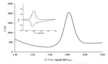
**Figure 2.** Square-wave voltammogram of  $4.31 \times 10^{-7}$  M HSA in 0.04 M B-R buffer at pH 7.4. (Inset: Cyclic voltammogram of  $4.31 \times 10^{-7}$  M HSA in 0.04 M B-R buffer (pH 7.4) at scan rate of 500 mVs<sup>-1</sup>). Other experimental conditions are described in the Procedure section.
