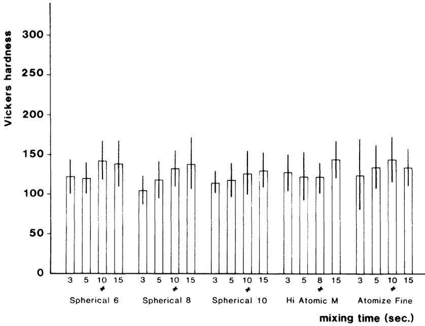
Figure 17 30-day Vickers hardness of low copper, spherical amalgams
