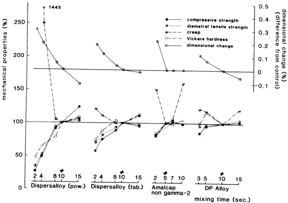
Figure 30 Comparison to manufacturer's recommended time; high copper, admixed amalgams
