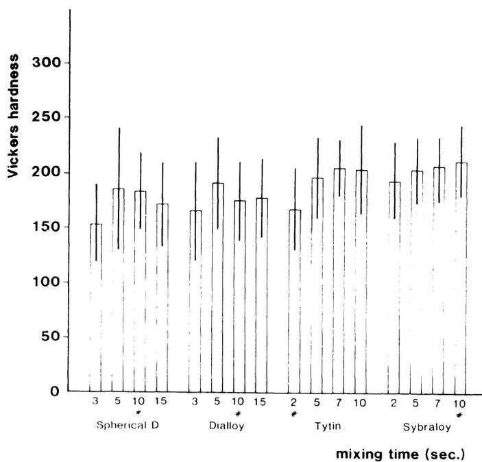
Figure 19 30-day Vickers hardness of high copper, single compositional amalgams
