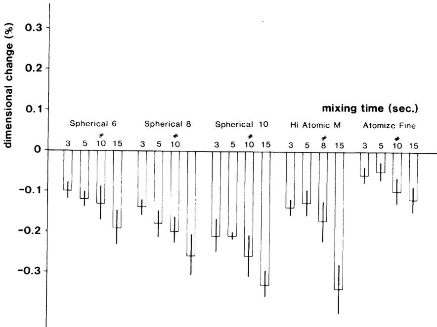
Figure 25 Dimensional change of low copper, spherical amalgams
