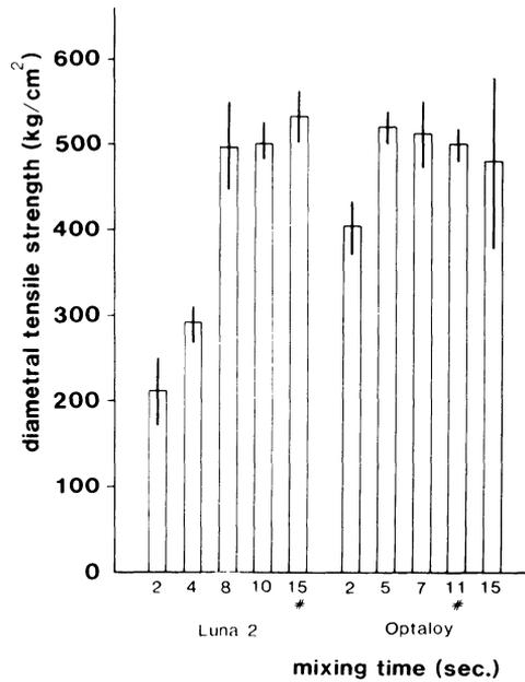
Figure 12 7-day diametral tensile strength of low copper, lathe-cut amalgams
