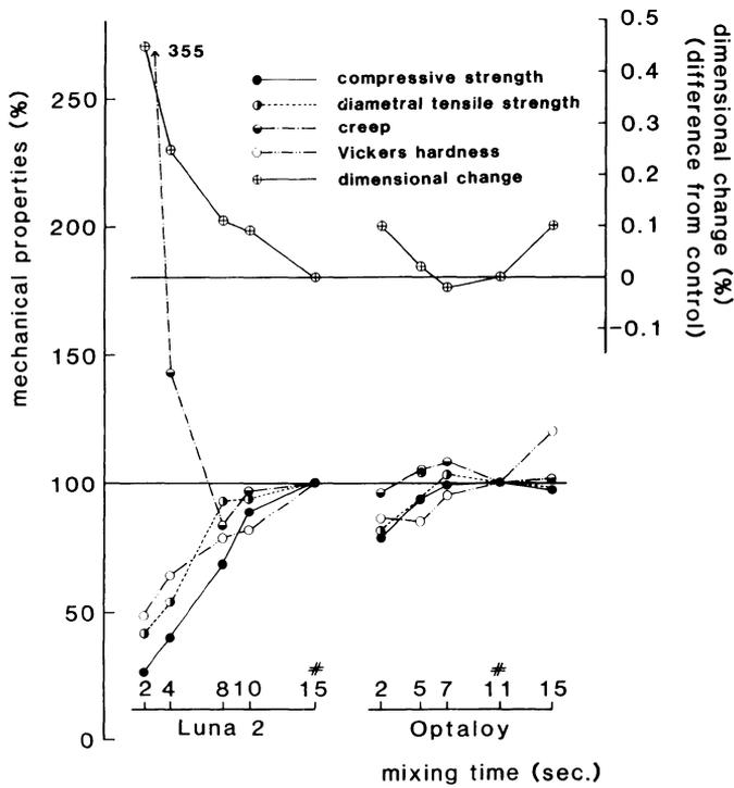
Figure 28 Comparison to manufacturer's recommended time; low copper, lathe-cut amalgams
