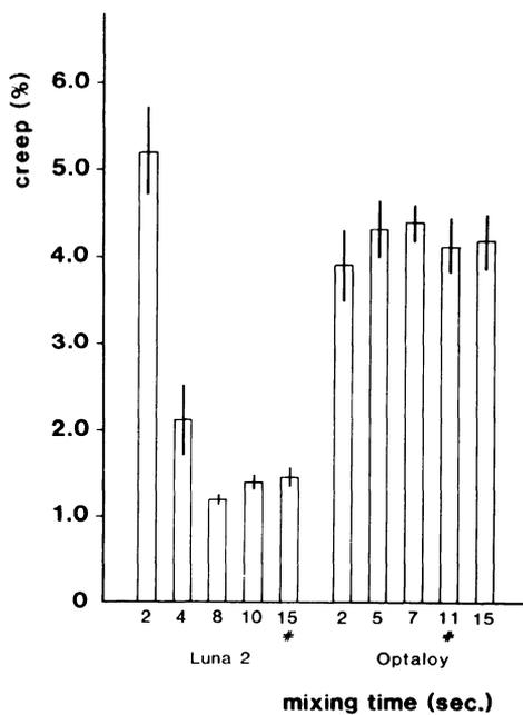
Figure 20 Creep of low copper, lath-cut amalgams
