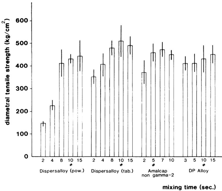
Figure 14 7-day diametral tensile strength of high copper, admixed amalgams
