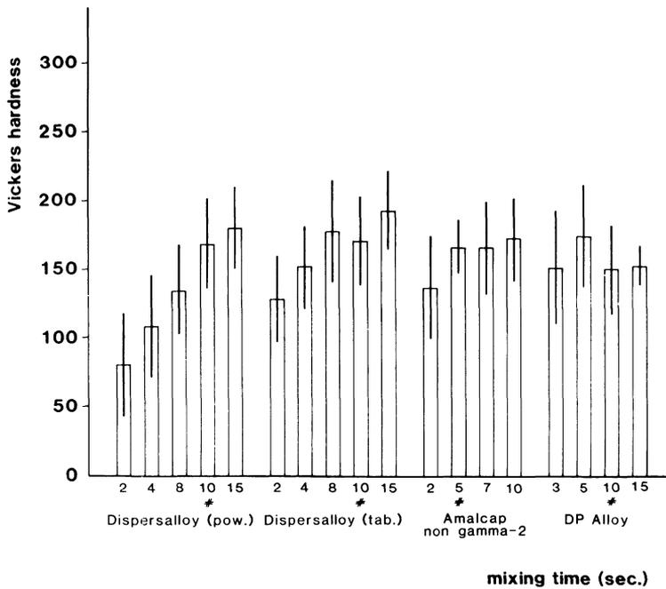
Figure 18 30-day Vickers hardness of high copper, admixed amalgams
