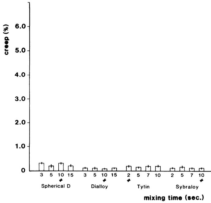
Figure 23 Creep of high copper, single compositional amalgams
