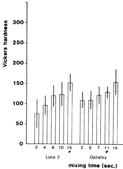
Figure 16 30-day Vickers hardness of low copper, lathe-cut amalgams
