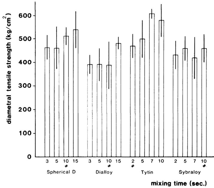
Figure 15 7-day diametral tensile strength of high copper, single compositional amalgams
