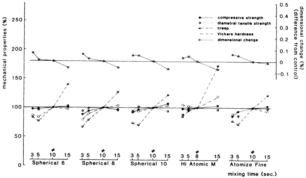
Figure 29 Comparison to manufacturer's recommended time; low copper, spherical amalgams
