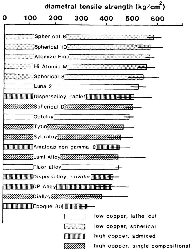
Fig. 3 7-day diametral tensile strength
