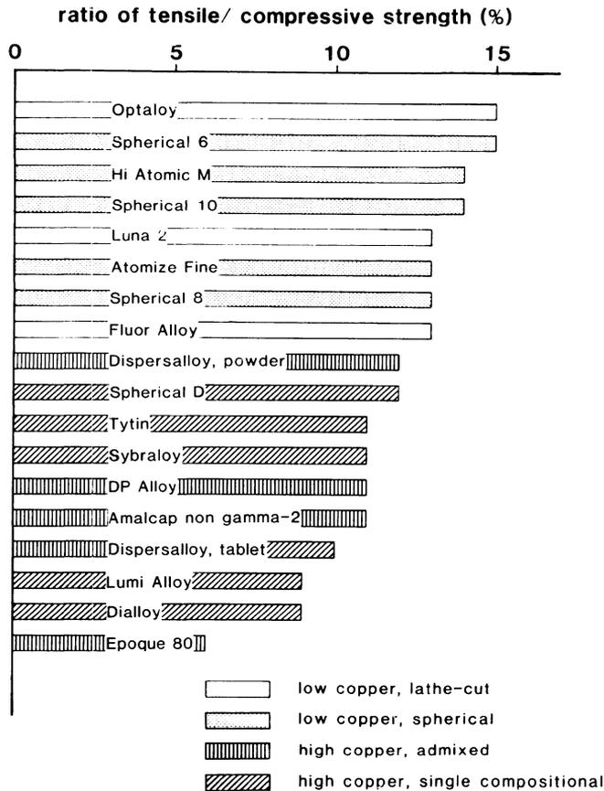
Figure 4 Ratio of 7-day diametral tensile to compressive strength
