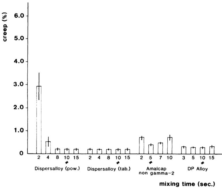
Figure 22 Creep of high copper, admixed amalgams
