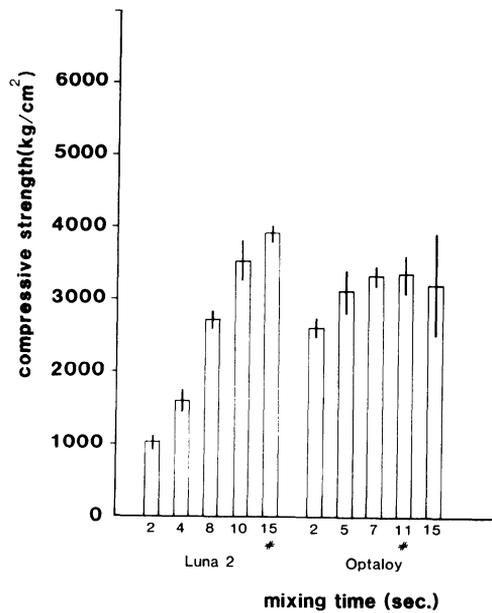
Figure 8 7-day compressive strength of low copper, lathe-cut amalgams
