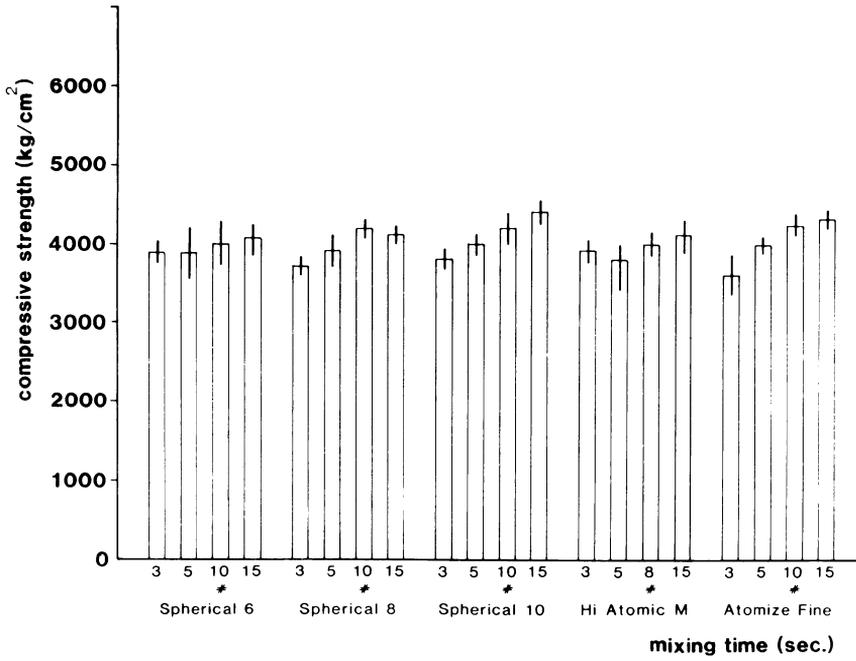
Figure 9 7-day compressive strength of low copper, spherical amalgams
