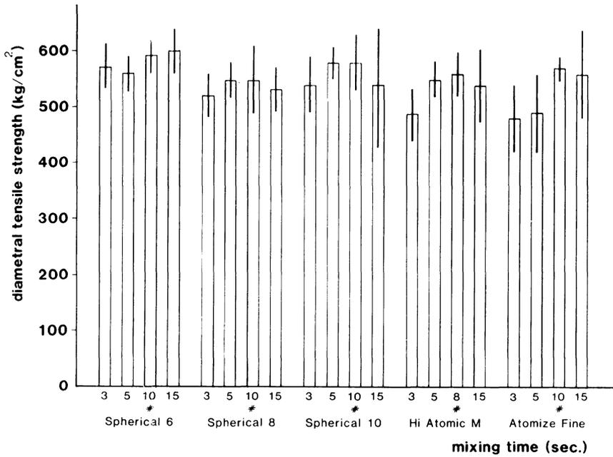
Figure 13 7-day diametral tensile strength of low copper, spherical amalgams
