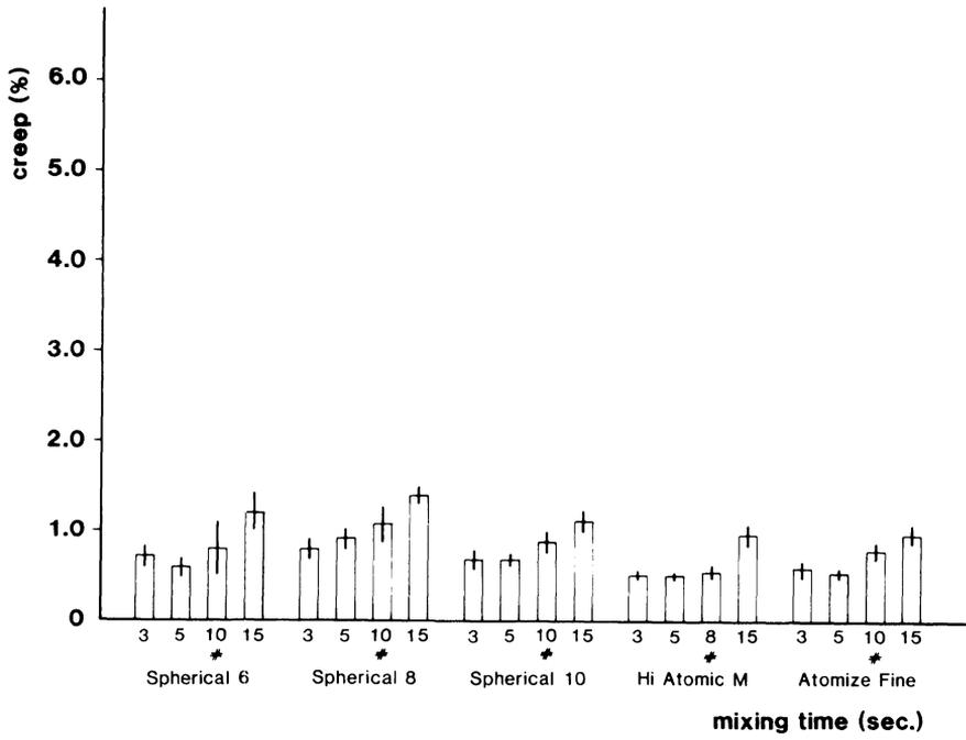
Figure 21 Creep of low copper, spherical amalgams
