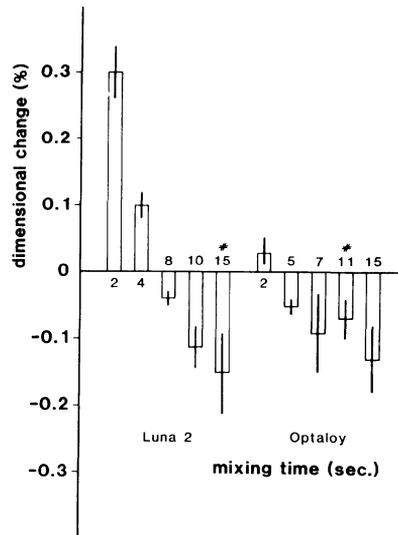
Figure 24 Dimensional change of low copper, lathe-cut amalgams
