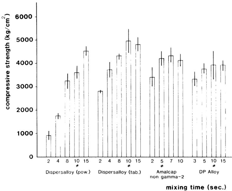
Figure 10 7-day compressive strength of high copper, admixed amalgams
