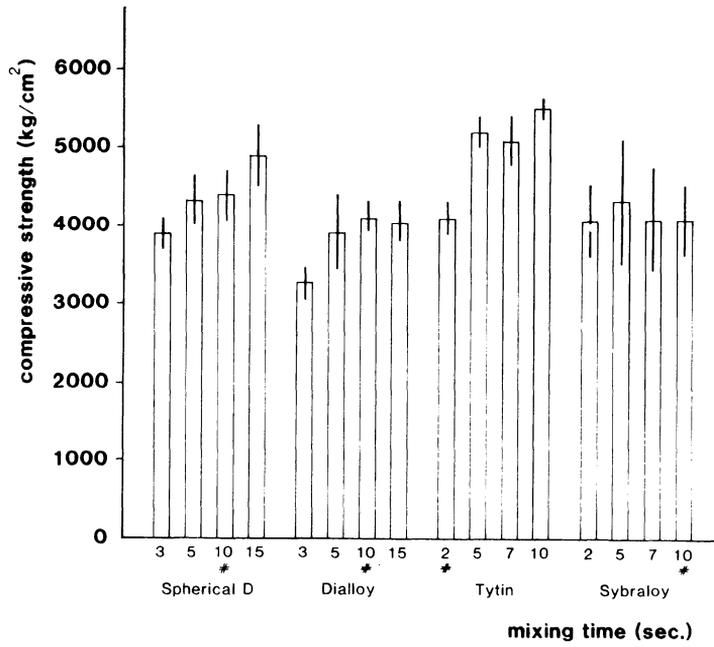
Figure 11 7-day compressive strength of high copper, single compositional amalgams
