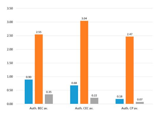
■ cost of water treatment €/m<sup>3</sup> ■ yield of struvite kg/m<sup>3</sup> of solution ■ cost of struvite €/kg
