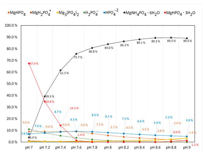
Figure 2. Phosphate speciation as a function of pH as determined by the MINEQL+ software.
