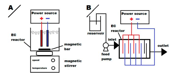
Figure 1. Reactor set-up for (A) batch electrocoagulation (BEC) and (B) continuous electrocoagulation (CEC) experiments.
