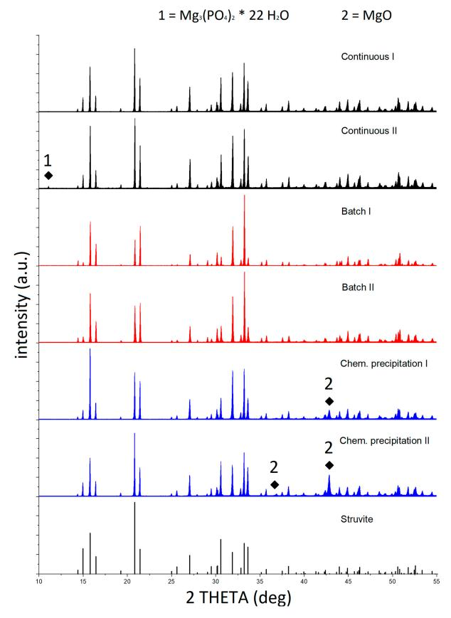
**Figure 4.** XRD patterns for the sludges obtained from the authentic water samples subjected to BEC, CEC, and CP for struvite precipitation.
