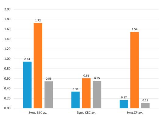
■ cost of water treatment  $\notin/m^3$  ■ yield of struvite  $kg/m^3$  of solution  $\equiv$  cost of struvite  $\notin/kg$
