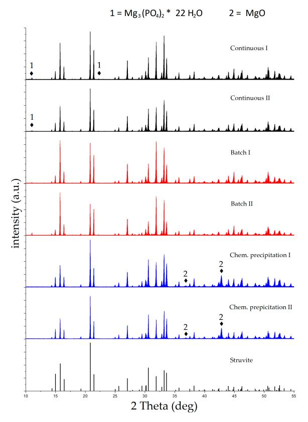
**Figure 3.** XRD (X-ray diffraction) patterns for the sludges obtained from the synthetic water samples subjected to BEC, CEC, and CP (chemical precipitation) for struvite precipitation.
