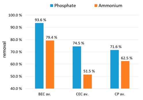
**Figure 5.** Average phosphate and ammonium removal (%) by BEC, CEC, and CP in synthetic water treatment. BEC av., Batch electrocoagulation average value; CEC av., continuous electrocoagulation average value; CP av., chemical precipitation average value.
