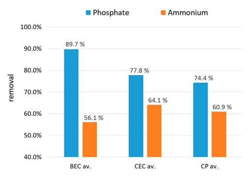
**Figure 6.** Average phosphate and ammonium removal rates of the BEC, CEC, and CP in authentic water treatment. BEC av., batch electrocoagulation average value; CEC av., continuous electrocoagulation average value; and CP av., chemical precipitation average value.
