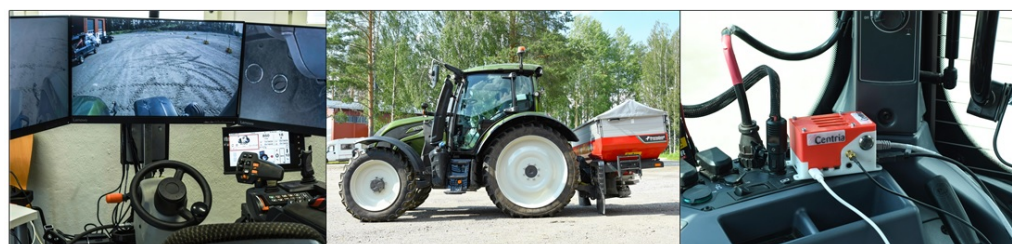
Figure 3. Elements of the remote-controlled tractor: the remote control cabin on the left, the remote-controlled tractor on the middle, and the computer for CAN tunneling over mobile networks on the right.
