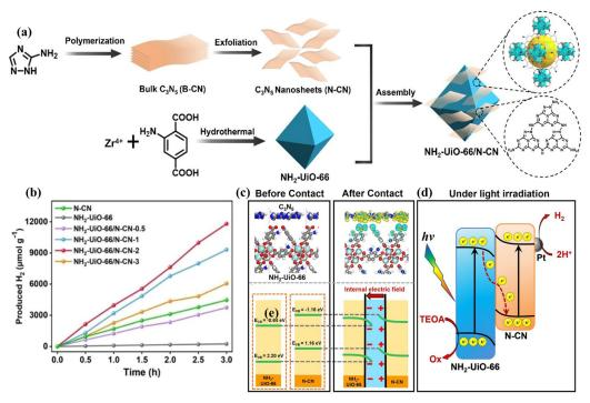
**Figure 13.** NH<sub>2</sub>-UiO-66/N-CN Z-scheme Heterojunction: (**a**) synthetic routes; (**b**) photocatalytic H<sub>2</sub> production amounts; (**c**) charge density differences and energy-level diagrams; (**d**) the proposed Z-scheme charge transfer mechanism. Adapted with permission from [52]. Copyright American Chemical Society, 2022.
