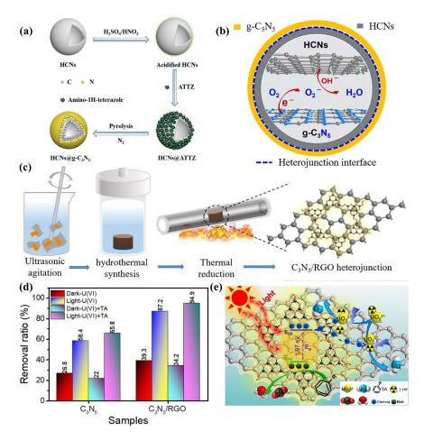
Fermi levels produced band bending and an internal electric field. They act similarly to a Schottky heterojunction to promote the separation of electrons and holes.
