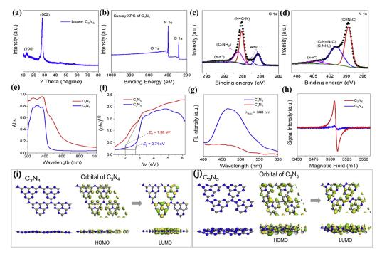
**Figure 3.** The characterization of  $g-C_3N_5$ : (a) XRD pattern; (b) XPS survey; (c) high-resolution C1s spectra; (d) high-resolution N1s XPS spectra for  $g-C_3N_5$ ; (e) UV–vis DRS; (f) Tauc's plot; (g) PL spectra; (h) ESR spectra for  $g-C_3N_5$  and  $g-C_3N_4$ ; (i, j) The orbitals for  $g-C_3N_4$  and  $g-C_3N_5$ . Adapted with permission from [28]. Copyright Elsevier B.V., 2021.
