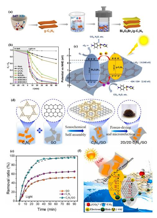
**Figure 12.** (a)  $g-C_3N_5/Bi_4O_5Br_2$  preparation routes; (b) Photocatalytic degradation of STZ by  $g-C_3N_5/Bi_4O_5Br_2$ ; (c) Photoreaction mechanism of STZ by  $g-C_3N_5/Bi_4O_5Br_2$ ; (d) Diagram of the  $g-C_3N_5/GO$  preparation; (e) U(VI) removal ratio; (f) Mechanism schematic of U (VI) extraction by  $C_3N_5/GO$ . (a–c) Adapted with permission from [42]. Copyright Elsevier B.V., 2021 (d–f) Adapted with permission from [56]. Copyright Elsevier B.V., 2021.
