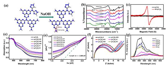
**Figure 9.** (a) Structures of  $g-C_3N_5$  and  $N_V-g-C_3N_5$ ; (b) FT-IR spectra; (c) ESR spectra; (d) UV-vis spectra; (e) Tauc's Plots; (f) EIS spectra; (g) FL spectra of  $g-C_3N_5$  and  $N_V-g-C_3N_5$  (0.01, 0.02, 0.05, 0.1, and 0.2 represent the amounts of NaOH for vacancy production). (b–f) Adapted with permission from [41]. Copyright American Chemical Society, 2020.
