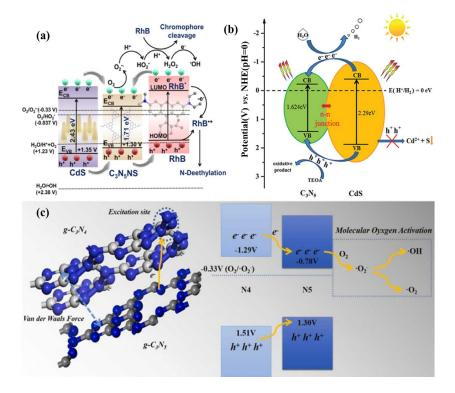
**Figure 11.** (a)  $CdS/C_3N_5$  for RhB degradation; (b)  $CdS/C_3N_5$  for H<sub>2</sub> evolution; (c) g-C<sub>3</sub>N<sub>4</sub>/g-C<sub>3</sub>N<sub>5</sub> for RhB and TC-HCl. (a) Adapted with permission from [53]. Copyright American Chemical Society, 2021. (b) Adapted with permission from [54]. Copyright Informa UK Limited, trading as Taylor and Francis Group, 2022. (c) Adapted with permission from [55]. Copyright Elsevier B.V., 2022.
