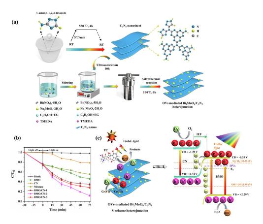
**Figure 14.**  $g-C_3N_5/Bi_2MoO_6$  S-scheme heterojunction: (**a**) synthetic routes; (**b**) photocatalytic degradation of TC; (**c**) S-scheme charge transfer mechanism. Adapted with permission from [45]. Copyright Elsevier Inc., 2022.
