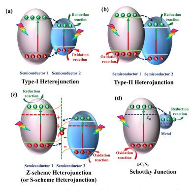
heterojunction or S-scheme heterojunction, and Schottky junction. Their photoinduced carrier transfer routes are shown in Figure 10.
