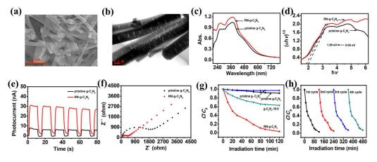
**Figure 5.** RN-g-C<sub>3</sub>N<sub>5</sub>: (a) SEM image; (b) TEM image; (c) UV–vis DRS spectra; (d) Tauc's plots; (e) The photocurrent response; (f) EIS spectra; (g) MB degradation; (h) Recyclability of g-RN-C3N5. Adapted with permission from [20]. Copyright American Chemical Society, 2019.
