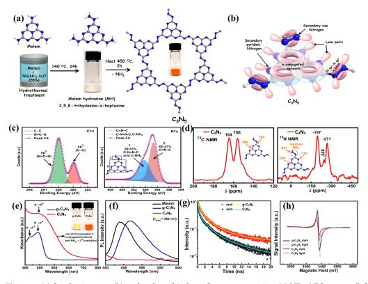
**Figure 6.** (a) Synthesis route; (b) molecular orbital overlap representation; (c) HR–XPS spectra (left: C1s, right: N1s); (d) CPMAS NMR spectra (left: <sup>13</sup>C, right: <sup>15</sup>N); (e) UV–vis spectra (blue:  $g-C_3N_4$ ; red:  $g-C_3N_5$ ); (f) steady state PL spectra; (g) PL lifetime decay curves; (h) X–band EPR spectra; Adapted with permission from [4]. Copyright American Chemical Society, 2019.
