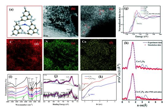
**Figure 7.** Co-C<sub>3</sub>N<sub>5</sub> (**a**) Doping structure; (**b**) HR-TEM image; (**c**) HAADF-STEM images; (**d**–f) elemental mapping; (**g**) XANES spectra; (**h**) R-space of XANES; (**i**) FT-IR spectra; (**j**) XPS spectra of Co<sub>2p</sub>; (**k**) Tauc's plot. (**a**–**h**) Adapted with permission from [32]. Copyright Royal Society of Chemistry, 2022. (**i**–**k**) Adapted with permission from [33]. Copyright Elsevier B.V., 2022.
