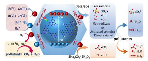
Figure 19. Photo-degradation processes of pollutants by g-C<sub>3</sub>N<sub>5</sub>-based materials.
