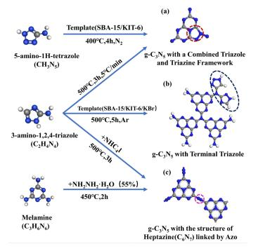
**Figure 1.** Schematic illustration of the  $g-C_3N_5$  synthesis process by the thermal polymerization of different precursors, such as 5-amino-1H-tetrazole, 3-amino-1,2,4-triazole, and melamine. (a)  $g-C_3N_5$  with triazine and triazole; (b)  $g-C_3N_5$  with terminal triazole; (c)  $g-C_3N_5$  with heptazine linked by azo.
