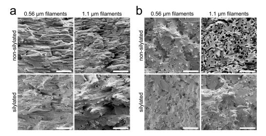
**Figure 6.** Composite morphology. Longitudinal (**a**) and transverse (**b**) fracture surfaces of the CNF filament/epoxy composites. (The scale bar is 5  $\mu$ m in all images.)
