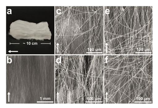
**Figure 3.** CNF filaments. (**a**) A photograph and (**b**) an optical microscope image of a CNF filament network. FESEM images of non-silylated (**c**) 1.1 and (**d**) 0.56  $\mu$ m and silylated (**e**) 1.1 and (**f**) 0.56  $\mu$ m filaments. The white arrow indicates the freezing direction.
