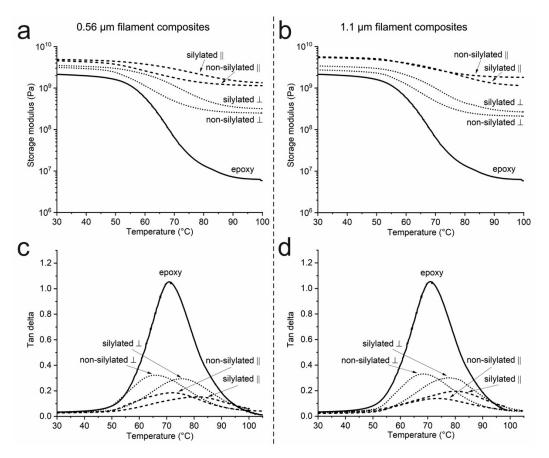
**Figure 8.** Viscoelastic properties of the CNF filament/epoxy composites. Storage modulus of the (a) 0.56 and (b) 1.1  $\mu$ m filament composites. Tan delta of the (c) 0.56 and (d) 1.1  $\mu$ m filament composites. Longitudinal (||) and transverse ( $\perp$ ) specimens were prepared from the composite samples.
