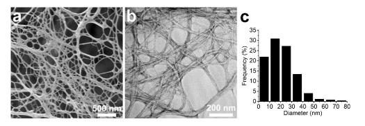
**Figure 2.** Cellulose nanofibers. (**a**) FESEM and (**b**) TEM images, and (**c**) the size distribution of the CNFs used as a raw material.
