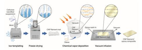
**Figure 1.** Process schematic. Ice-templating was used to orient the cellulose nanofibers (CNFs) into thin filaments, and dry filament mats were obtained after freeze-drying. The filament surfaces were covered with an aminosilane, and the treated filament mats were impregnated with a bio-epoxy resin to form composites.
