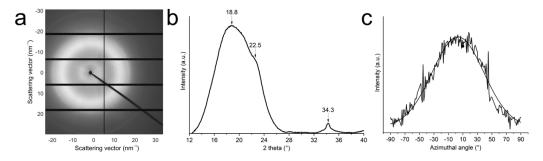
**Figure 7.** Analysis of filament alignment in the composites using 2D-WAXS. The meridional direction coincides with the freezing direction during ice-templating, i.e., the filament direction. (a) A representative diffractogram of a 1.1  $\mu$ m filament/epoxy composite. (b) Radial integration of the diffractogram after baseline subtraction. (c) Azimuthal integration of the (004) plane. The zero degree was set on meridian.
