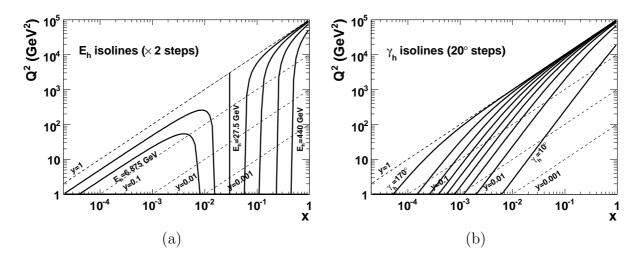
Figure 5.5: Isolines of the hadronic system's energy,  $E'_h$ , and polar angle,  $\gamma_h$  in the x-Q<sup>2</sup> kinematic plane [118]. The dashed lines in the background indicate isolines for the kinematic variable y.
