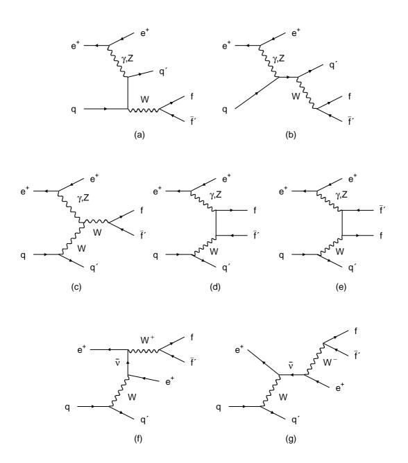
Figure 2.9: Main Feynman diagrams for single W production: (a) and (b) are the dominant diagrams, (c) involves a triple gauge coupling, (d) and (e) contain off-shell W bosons, (f) and (g) contain a second W propagator and are therefore suppressed.
