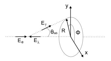
Figure 3.4: Compton scattering of an incident photon with energy  $E_{\lambda}$  off an electron with energy  $E_e$ . The scattered photon travels with energy  $E_{\gamma}$  in the direction specified by  $\theta_{\text{lab}}$  and  $\phi$ .
