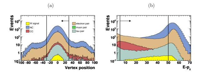
Figure 6.1: Distribution of MC events in the isolated electron search for the quantities  $Z_{\text{vtx}}$  and  $E - p_z$ . The the W signal MC only comprises the electron decay channel of the W boson in these plots.
