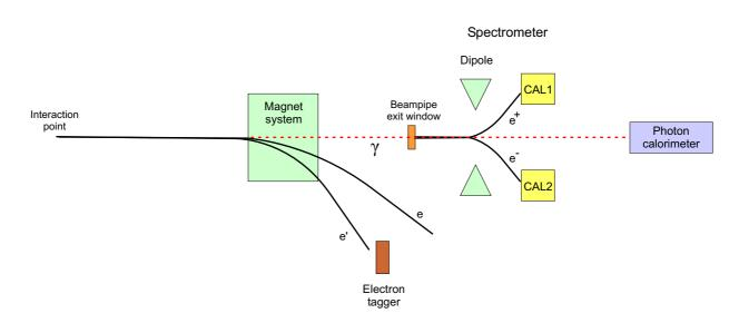
Figure 3.10: Diagram of the luminosity measuring devices: the original photon calorimeter plus 'electron tagger' and the spectrometer consisting of the dipole magnet and the two calorimeters, CAL1 and CAL2.
