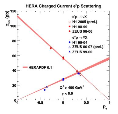
Figure 2.3: Measurements with the ZEUS and H1 detectors of the Charged Current cross section with  $e^+p$  (blue) and  $e^-p$  (red) data versus lepton beam polarisation  $P_e$  in the region of y < 0.9and  $Q^2 > 400 \text{ GeV}^2$  [24]. The straight bands indicate the corresponding SM prediction and the uncertainty on it from the parton density functions.
