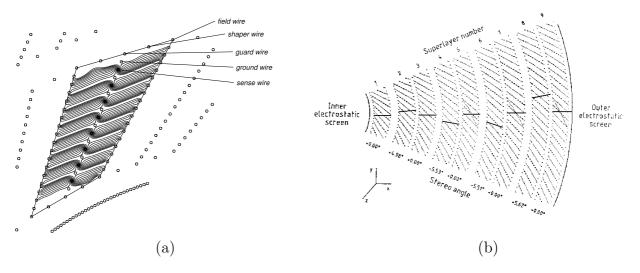
Figure 3.7: (a) Distribution of wires and the resultant field in a CTD cell. (b) The nine super-layers of the CTD with cells inclined by the Lorentz angle.
