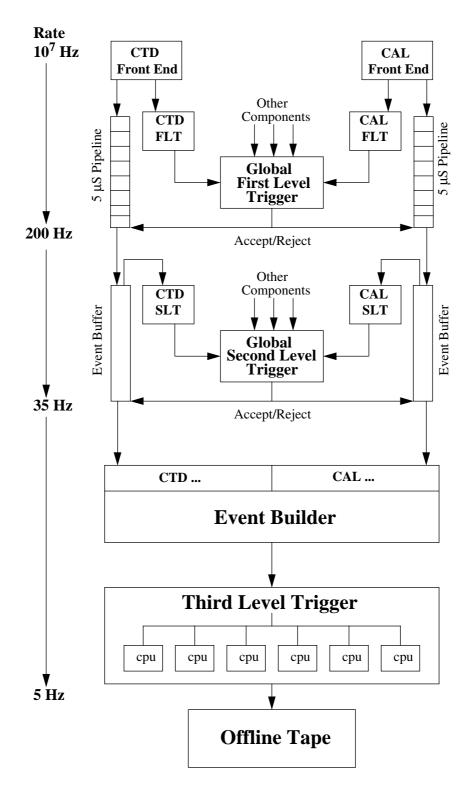
Figure 3.11: The ZEUS three-level trigger system [74] and the in- and output rates at every level. Only the two main components of the ZEUS detector, CTD and CAL, are shown in detail, but other components that feed into the global trigger levels are similar. The CTD SLT was replaced by the Global Tracking Trigger (GTT) in 2006 [75].
