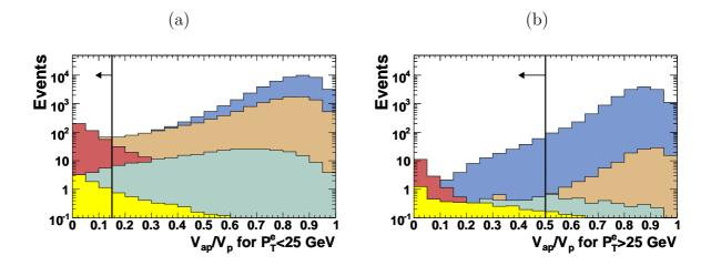
Figure 6.4: Distribution of MC events in the isolated electron search for the quantity  $V_{\rm ap}/V_{\rm p}$  below and above the  $P_T^e$  threshold. The W signal MC only comprises the electron decay channel of the W boson in these plots. The legend of Fig 6.1 applies.
