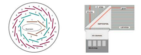
Figure 3.9: Layout of the MVD ladders around the beampipe in the cross sectional view (left) and an MVD half-module showing the  $r-\phi$  and r-z strips (right).
