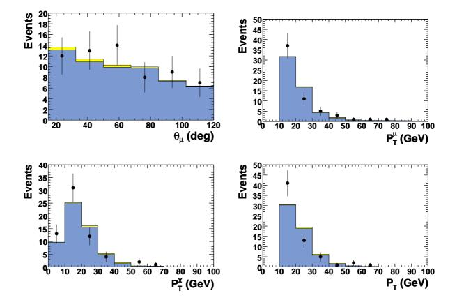
Figure 6.16: Distributions of the polar angle and transverse momentum of the muons, as well as the hadronic transverse momentum and total missing transverse momentum in the data and MC samples enriched with lepton pair production.
