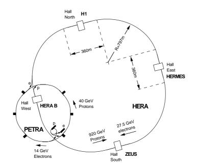
Figure 3.1: The HERA ring collider with the four experiments H1, HERMES, HERA-B and ZEUS and the pre-accelerator PETRA.
