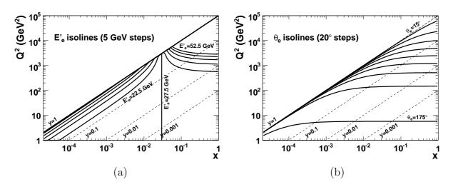
Figure 5.3: Isolines of the scattered electron's energy,  $E'_e$ , and polar angle,  $\theta_e$  in the x-Q<sup>2</sup> kinematic plane [118]. The dashed lines in the background indicate isolines for the kinematic variable y.
