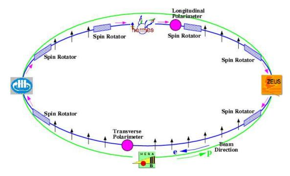
Figure 3.3: The position of the longitudinal and transverse polarimeter and the spin rotators around the experiments on the HERA ring. The direction of the lepton spin is indicated with black (transverse) and pink (longitudinal polarisation) arrows.
