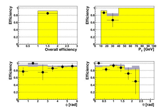
Figure 6.17: The efficiency of finding a muon with MV versus the azimuthal ( $\phi$ ) and polar angle ( $\theta$ ), as well as the transverse momentum of the muon ( $P_T$ ). The top left plot is the efficiency overall. The points indicate the efficiency in data, whereas the yellow histograms with violet error bands indicate the efficiency in MC.
