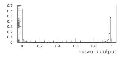
Figure 5.1: The muon finder output,  $P_{\mu}^{\text{MV}}$ , for MC samples of  $4 \times 10^5$  hadrons (filled histogram) and muons, respectively, with initial energy uniformly distributed in the region of 1–40 GeV [111]. The scale on the vertical axis is arbitrary.
