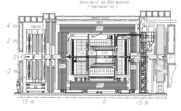
Figure 3.5: A cross sectional view of the ZEUS detector highlighting its subcomponents. The human on the left is drawn to indicate the scale.
