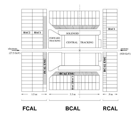
Figure 3.6: The sub-divisions of the ZEUS calorimeter.
