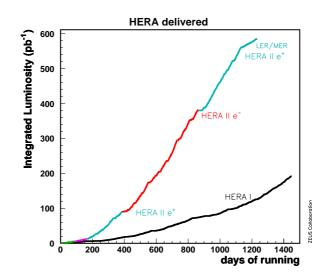
Figure 3.2: The luminosity delivered by HERA over the period 1992–2007. Run periods are split into high energy runs, denoted by HERA I and II, as well as medium (MER) and low energy runs (LER).
