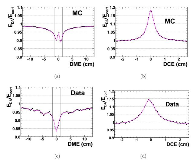
Figure 5.6: The mean of the Gaussian fit to the  $E_{DA}/E_{cor1}$  distribution versus (a) DME and (b) DCE for positrons in Monte Carlo and correspondingly for data in (c) and (d) [120]. The error bars on the points represent the error on the Gaussian mean and are smaller than the marker size.
