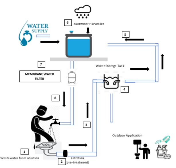
Figure 1: Model of Sharia Compliance Membrane Water Treatment
