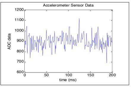
Fig. 1.Unfiltered accelerometer result of unmoving robot
