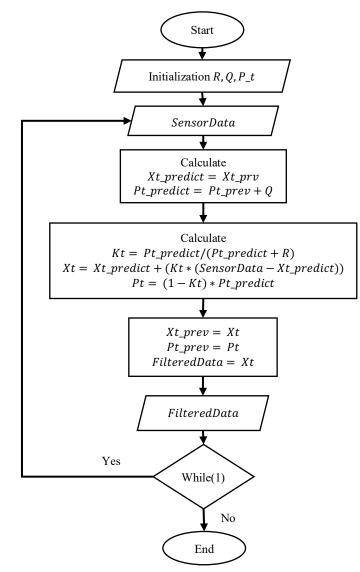
Fig. 2. Kalman Filter Flow Chart
