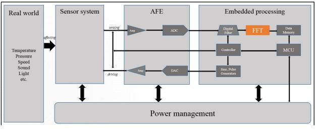
Figure 3 : Position of FFT module in an overall digital system.
