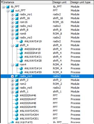
Figure 10: List of instances of proposed FFT processor.
