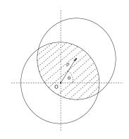
FIG. 4 Schematic representation of the autocorrelation function  $P * *_{corr} P$  of a nonuniform pupil function P as an integral over the common region of two disks of unit radius with centers at o and  $\rho e^{i\theta}$ , respectively.
