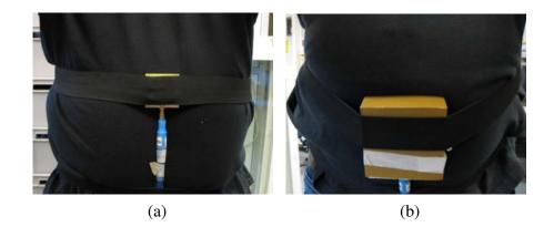
Figure 18. On-body measurement setup using the proposed UWB antenna (a) without and (b) with cavity.
