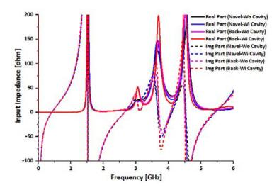
Figure 13. Simulated input impedance of the UWB antenna with and without the cavity close to Navel and Back regions of the voxel model.
