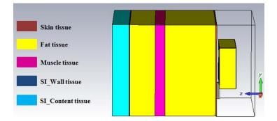
Figure 9. Abdominal multi-layer model used in simulations.
