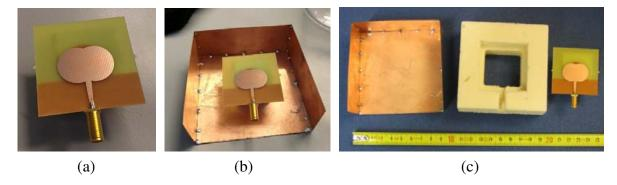
**Figure 4.** UWB antenna prototype (a) without and (b) with the cavity, (c) the three elements of the proposed antenna with cavity for on-body use.
