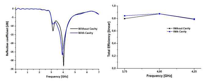
**Figure 1.** Simulated reflection coefficient of the UWB antenna with and without the cavity.
