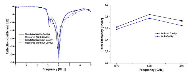
Figure 6. Simulated and measured reflection coefficient of the UWB antenna with and without cavity.
