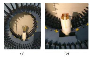
**Figure 5.** Setup for radiation patterns measurements, in free-space, using (a) horn antenna for calibration and (b) the proposed UWB antenna with cavity.
