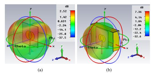
**Figure 3.** Simulated directivity (3D overview) of the UWB antenna at 4 GHz (a) without and (b) with the cavity in free-space.
