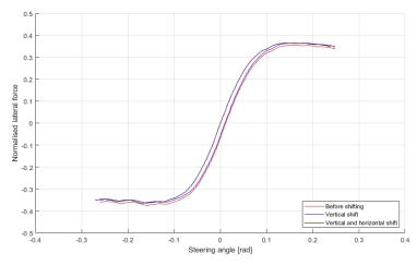
Figure 7. Elimination of lateral force curve shift caused by tyre conicity, ply-steer etc.
