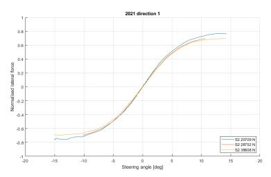
Figure 10. Pure lateral slip force curves of "S2" tyre on wet asphalt.
