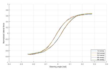
Figure 9. Individual sweeps of pure lateral force test run in wet asphalt with normal force of 39829 N.
