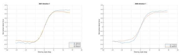
Figure 8. Comparison of "S2" tyre on snow in years 2021 and 2020.
