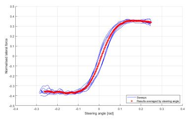
Figure 6. Relaxation compensation for the normalized lateral force curve.
