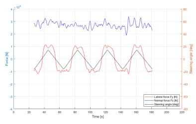
Figure 4. Filtered lateral and normal forces with steering angle in time domain for the 4 full sweeps of the test run.
