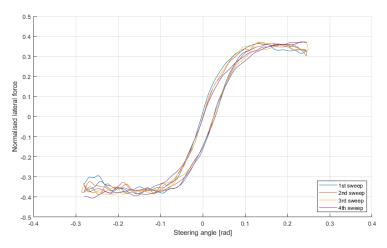
Figure 5. Normalized lateral force curves as a function of steering angle separated to individual sweeps of the measurement run.
