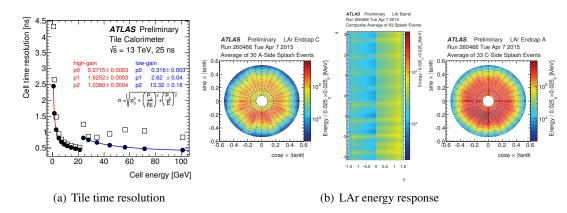
**Figure 4:** (a) Tile cell time resolution in jet events [4]. (b) LAr energy response uniformity in beam splash events [3], with an eight-fold banding pattern corresponding to shadows from the toroid magnets.
