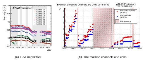
**Figure 3:** (a) Measured impurity of the liquid argon in the barrel cryostat [3]. (b) The percentage of all cells and channels in the Tile Calorimeter that are masked [4].
