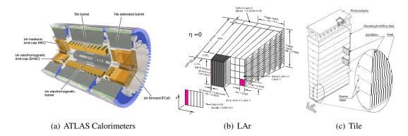
**Figure 1:** The ATLAS calorimeter systems (a) [2] consist of the Liquid Argon Calorimeter (b) [3] and the Tile Calorimeter (c) [4].
