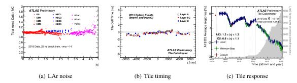
**Figure 2:** (a) Ratio of total noise in LAr (electronics and pile-up for  $\langle \mu \rangle = 14$ ) at the electron scale (data/MC) [3]. (b) Timing of Tile Calorimeter signals recorded with single beam data on April 2015 [4]. (c) The variation of the response to Minimum Bias, Cesium and Laser for cells in the inner layer of the Extended Barrel, covering the region  $1.2 < |\eta| < 1.3$ , as a function of time [4].
