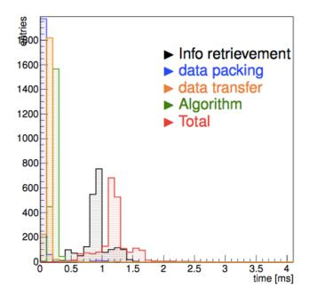
**Figure 1:** Time sharing of the different steps necessary to execute the *mulso* algorithm on a GPU using the *APE* interface
