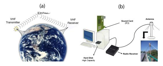
Figure 1: RMS method: (a) the detection principle and (b) the detector setup.
