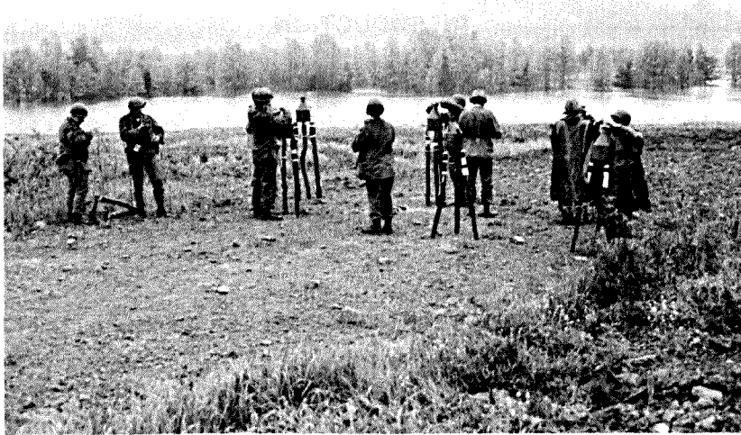
Figure A1. Shaped charges with wooden tripods used to obtain or achieve 48-in. standoffs
