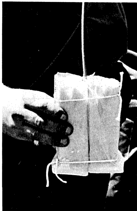
Figure 4. C-4 booster with detonator cord primer prior to loading downhole
