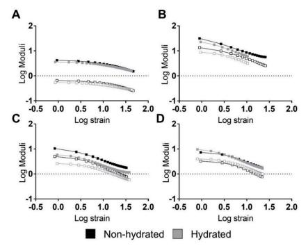
**Figure 3.** Strain sweeps of the studied PUs revealing strong relations between moduli and strain. Representative performances of hydrated and non-hydrated PUs: (**A**) 5–90–5, (**B**) 45–45–10, (**C**) 46.3–46.3–7.5, and (**D**) 47.5–47.5–5. Filled squares represent the storage modulus while non-filled squares represent the loss modulus.
