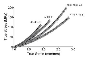
**Figure 6.** Hyperelastic modeling of true stress and true strain from synthesized PUs. Gray filled symbols represent the mean curve while the dashed line represents the hyperelastic model.
