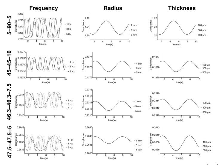
Figure 7. Response of PU-based vascular grafts under simulated physiological mechanical conditions. Compliance given in  $mmHg^{-1} \times 10^4$ .
