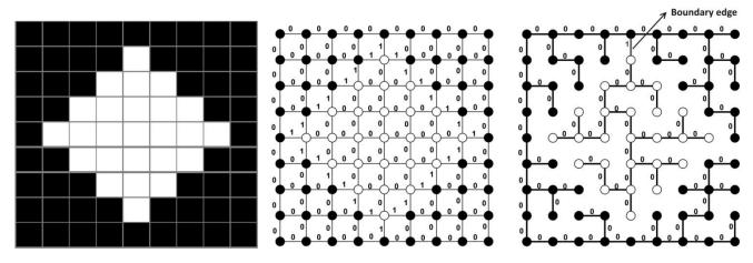
Figure 1. (a) A simple black and white image , (b) the graph representation of the image according to 4-connection neighborhood, (c) the MST of the image extracted from its graph representation and an example of boundary edge in the MST
