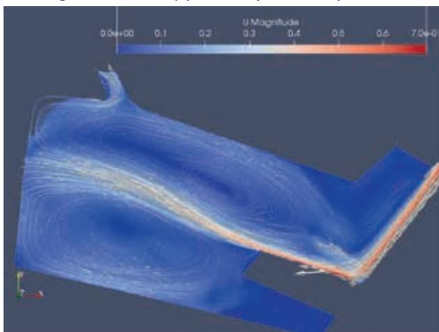
Figure 12: Velocity field at a flow rate of  $70 \text{ m}^3/\text{s}$
