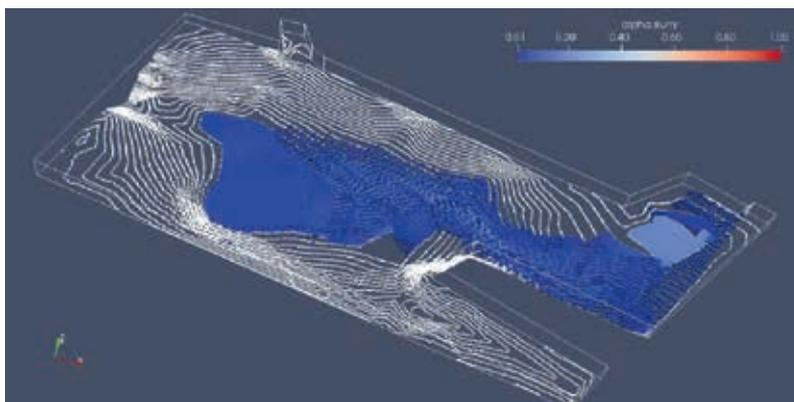
Figure 8: Sediment deposition area at a flow rate of  $35 \text{ m}^3/\text{s}$
