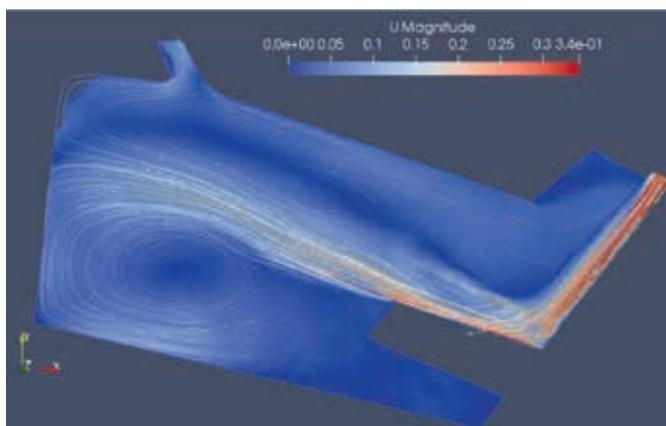
Figure 11: Velocity field at a flow rate of  $35 \text{ m}^3/\text{s}$
