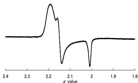
**Fig.2** Frozen solution EPR spectrum of the oxidized form of complex **8**. The sample was prepared in acetone solution (5 mM) by oxidizing at 195 K using 1 eq. of  $[Ce(NH_4)_2(NO_3)_6]$  as oxidizing agent.
