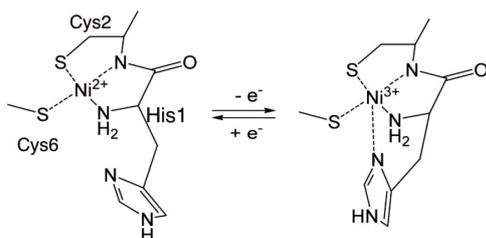
**Scheme 1.** Schematic structures of NiSOD active site in the reduced (left) and oxidized states (right).
