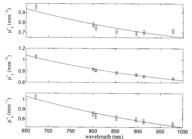
Fig. 5. Determination of broadband  $\mu'_s$  spectra for the three breast samples. Circles, the discrete  $\mu'_s$  values measured by the FD technique; solid curves, best power-law fits to Eq. (4). Fitting parameters ( $A, B$ ) from top to bottom are (240, -0.86), (2700, -12), and (250, -0.85). Error bars on  $\mu'_s$  are 3%.<sup>7</sup>
