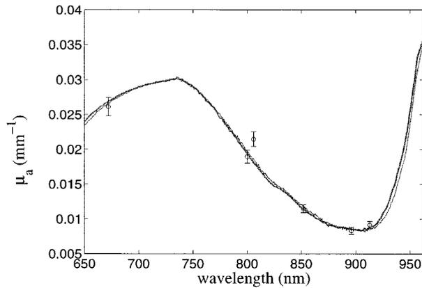
Fig. 6. Comparison of  $\mu_a$  values generated by FD (open circles) and by SSFD (thicker curve) for the dye-Intralipid phantom. Also shown is the best fit (thinner curve) to the SSFD data by use of the spectra of naphthol (measured with a spectrophotometer) and of water (from Kou *et al.*<sup>26</sup>). Open circles, discrete  $\mu_a$  values from FD alone. Error bars,  $\pm 0.0005 \text{ mm}^{-1}$  or 5%, whichever is larger.
