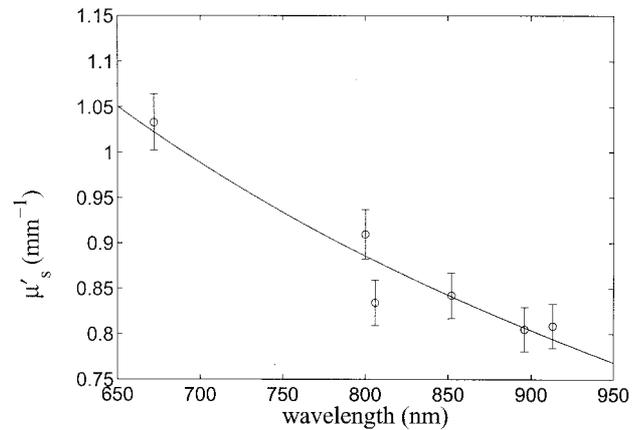
Fig. 4. Determination of the broadband  $\mu'_s$  spectrum for the dye-Intralipid phantom. Open circles, discrete  $\mu'_s$  values measured by the FD technique; solid curve, best power-law fit to Eq. (4). Fitting parameters are  $A = 2200$  and  $B = -0.82$ . Error bars on  $\mu'_s$  are 3%.<sup>7</sup>
