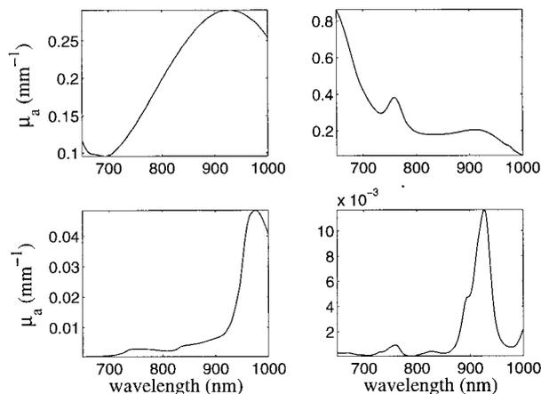
Fig. 10. Absorption spectra of major absorbers in breast tissue. Upper left, oxyhemoglobin, 1  $\mu\text{M}$ ; upper right, deoxyhemoglobin, 1  $\mu\text{M}$ ; lower left, water, 1  $\text{g}/\text{cm}^3$ ; lower right, fat (soybean oil), 0.9  $\text{g}/\text{cm}^3$ . The hemoglobin spectra are from Wray *et al.*,<sup>27</sup> the water is from Kou *et al.*,<sup>26</sup> and the fat is from the doctoral dissertation of Eker.<sup>28</sup>
