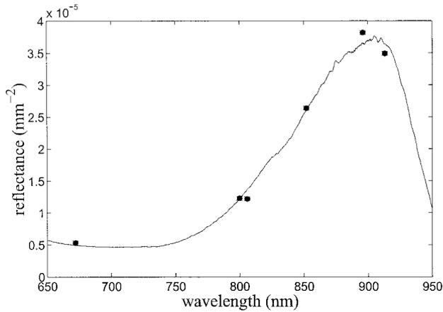
Fig. 2. SS reflectance spectrum acquired from a dye-Intralipid phantom, scaled to fit the discrete reflectance values (filled circles) predicted by Eqs. (1) and (2) with FD-derived values of  $\mu'_s$  and  $\mu_a$ . This scaling causes the entire spectrum to be converted into absolute reflectance units; see text for a discussion. The error in FD reflectance is estimated to be  $\pm 3 \times 10^{-7}/\text{mm}^{-2}$ ; in SS reflectance,  $\pm 1 \times 10^{-7}/\text{mm}^{-2}$ .
