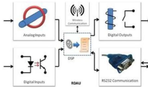
Fig. 2: RDAU block diagram.
