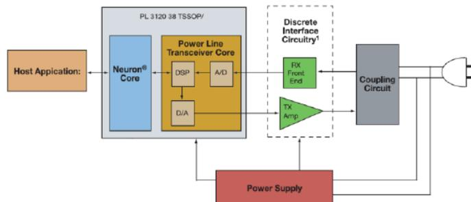
Fig. 8: PLC node based in PL-3120.
