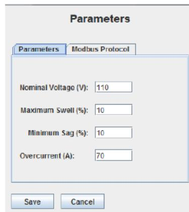
The image shows a software dialog box titled "Parameters". It has two tabs: "Parameters" (selected) and "Modbus Protocol". The "Parameters" tab contains four input fields with the following values: "Nominal Voltage (V): 110", "Maximum Swell (%): 10", "Minimum Sag (%): 10", and "Overcurrent (A): 70". At the bottom of the dialog are two buttons: "Save" and "Cancel".
