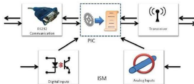
Fig. 5: ISM block diagram.
