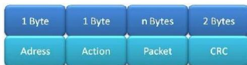
Fig. 7: MODBUS RTU framing.
