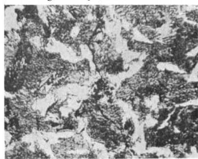
Fig. 19. Swedish Iron, Fractured at 1 Blow.
