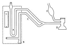
The U-tube and escape valve are assembled on a plastic board fitted with a Gabler snaplock to fit a Gabler wall rail. The Bennet face mask is applied snugly to the patient's face. The constant positive pressure is adjusted according to the needs of the patient.
