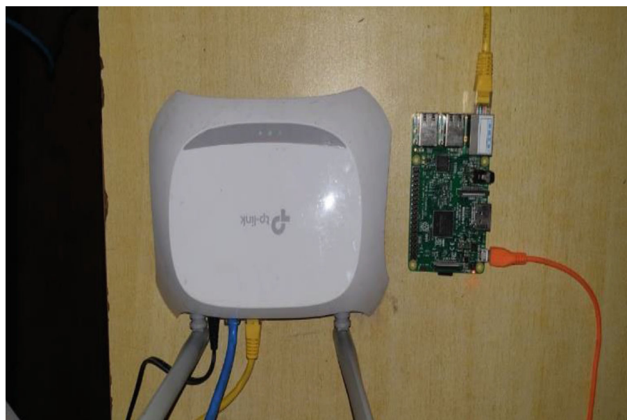
FIGURE 9: Raspberry Pi server and router setup.
