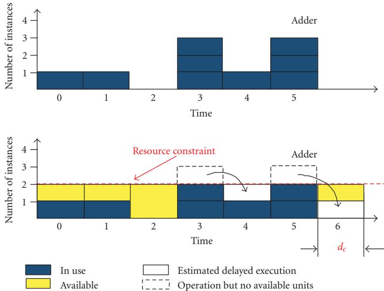
FIGURE 5:  $d_c$  Computation for given resource constraint.
