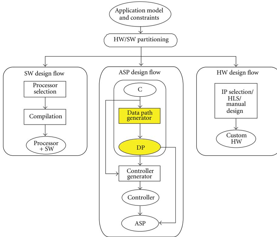
FIGURE 1: Proposed design technique within system-level design flow.
