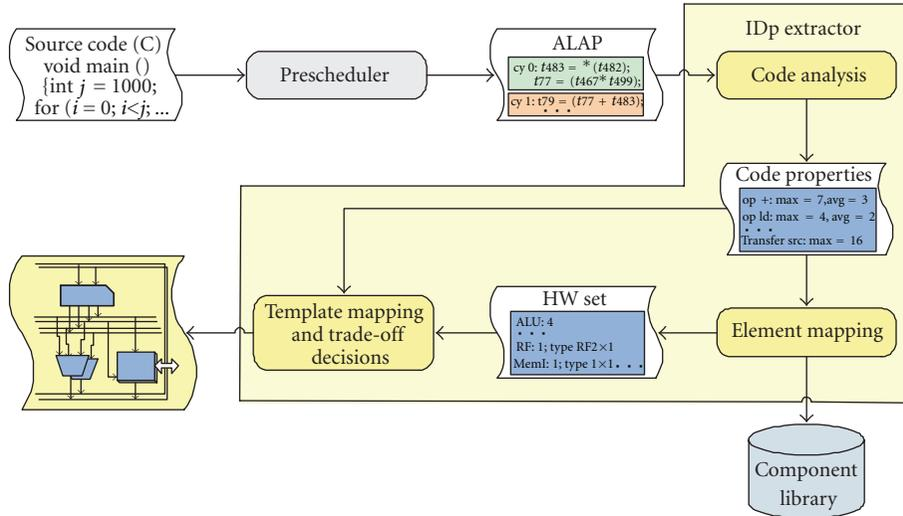
FIGURE 4: Initial data path (IDp) extraction flow.
