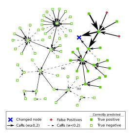
Figure 2: An illustration of impact prediction based on weighted call graphs. Edges with a low weight (< 0.2) are considered as non-propagating the impact of the change.
