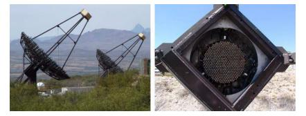
Figure 8. Left: The first two VERITAS Telescopes. Right: The 499 pixel PMT camera.
