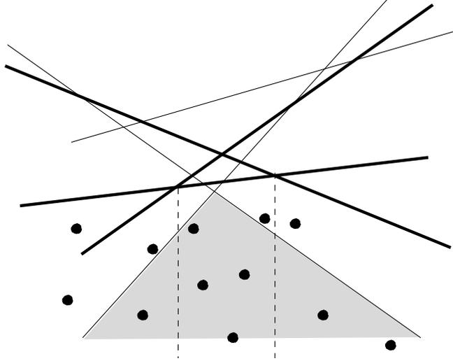
Figure 1: A planar point set and a collection  $\Gamma$  of upper halfplanes. A random sample of the lines bounding these halfplanes is shown in bold, with a decomposition of the region below their lower envelope, which contains the region below the lower envelope of all the bounding lines, drawn shaded.
