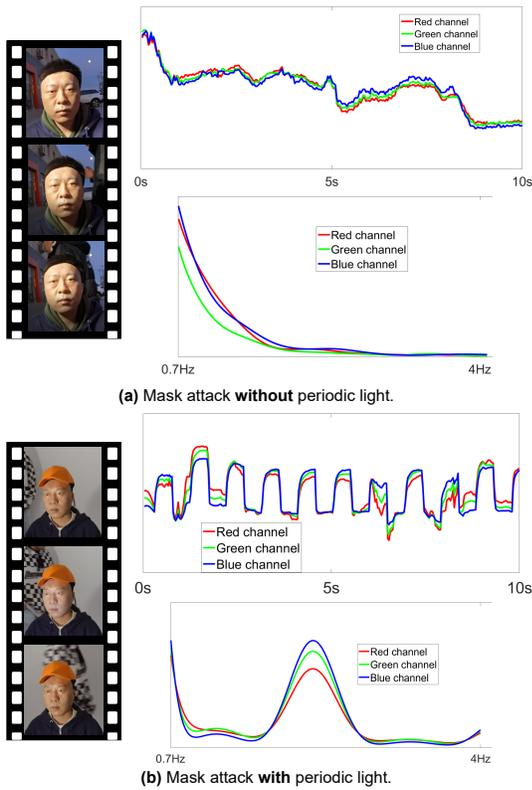
Fig. 7. Visualization of video samples and their extracted rPPG signal and power spectral density (PSD). In both cases, i.e., without (a) and with (b) external periodic light, the top right sub-figures illustrate the rPPG signal in time domain while the bottom right ones show their PSD in frequency domain. It can be seen from (b) that with period light, mask attacks could also contain pseudo ‘live’ pulse clues. **Best viewed in color.**
