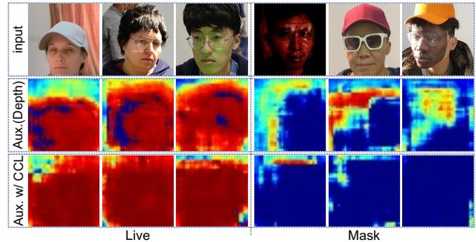
Fig. 9. Visualization of several samples in HiFiMask. The maps are performed from Aux.(Depth) in the second row and Aux. w/ CCL in the third row (Red color: the higher the better for live samples; Blue color: the higher the better for mask samples.). **Best viewed in color.**
