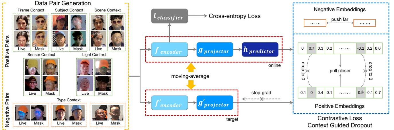
Fig. 4. The CCL framework. The left part (yellow) denotes our data pair generation manner. Each pair of images is processed by central framework twice, consisting of an online network ( $f$ ,  $g$ ,  $h$ ), a target network without gradient backward ( $f'$ ,  $g'$ ) and a classifier header ( $l$ ). The right part (blue) denotes the CGD module, the positive embeddings are pulled closer by CGD.
