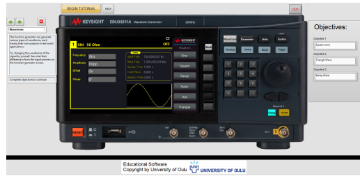
Fig. 8: VI of a function generator (Keysight EDU33211A)
