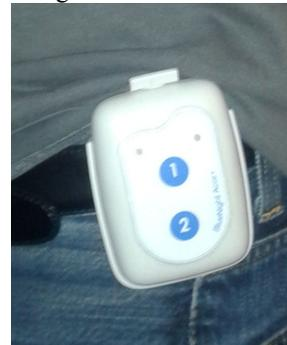
**Figure 1. The ACOR+ is an IMU with reduced dimensions (77x57x25 mm) and light weight (70 g) to be clipped on the belt.**
