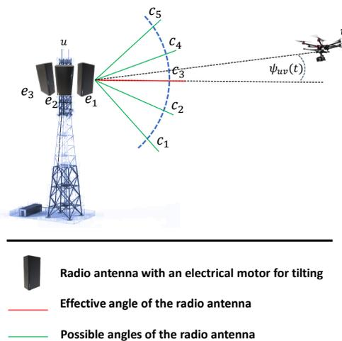
Fig. 1: Tilting the radio antenna: a radio antenna with an electrical motor can take several positions by tilting its angle.
