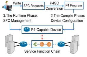
Fig. 11. A service function chaining framework on P4-enabled devices [170].
