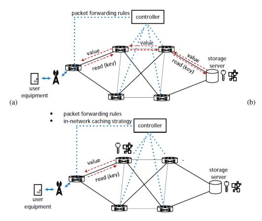
Fig. 7. (a) Caching system in general, (b) In-network caching.
