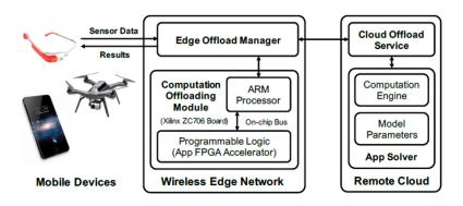
Fig. 8. Computation at edge enhanced with FPGA accelarator [144].
