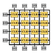
Fig. 5. FPGA architecture. [45].
