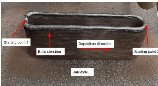
Fig. 1. Diagram of the WAAM printed part. The printing directions and starting points for printing are shown in the figure.
