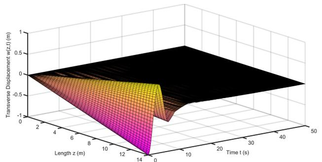
**FIGURE 3. Case I: transverse displacement of the HDS with the proposed control scheme.**
