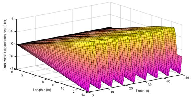
**FIGURE 2. Transverse displacement of the HDS without controller.**
