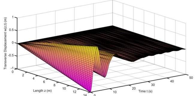
FIGURE 10. Case II: transverse displacement of the HDS with the control scheme neglecting backlash [12].
