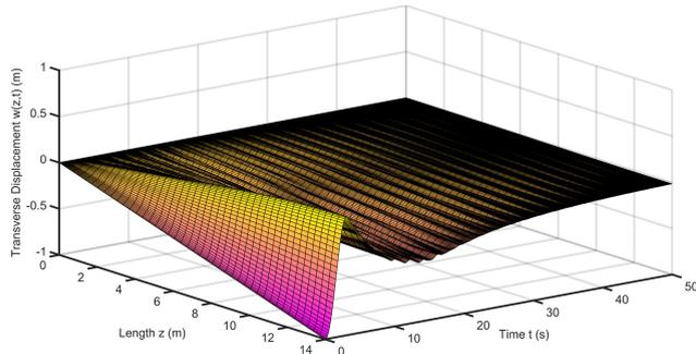
FIGURE 4. Case I: transverse displacement of the HDS with the control scheme neglecting saturation [13].
