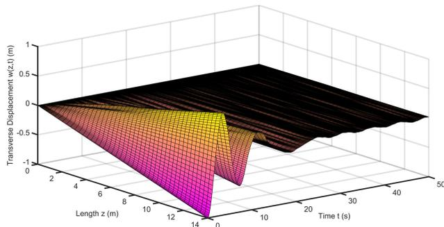
FIGURE 5. Case I: transverse displacement of the HDS with the control scheme neglecting dead-zone [12].
