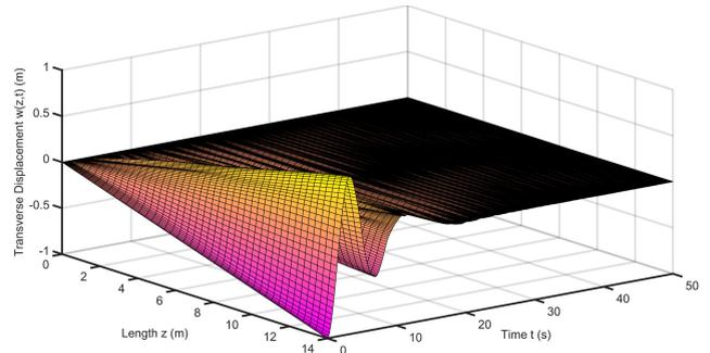
FIGURE 8. Case II: transverse displacement of the HDS with the proposed control scheme.
