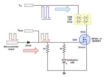
Fig.7. Design of the LED driver circuit arrangement.
