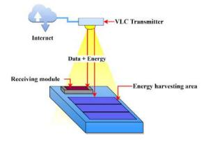
Fig.1. Structure of LIoT device
