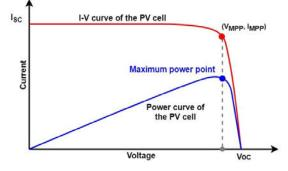
Fig.2. I-V curve of a PV cell.
