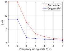
Fig.16. Frequency vs SNR variation of perovskite and organic PV cells.
