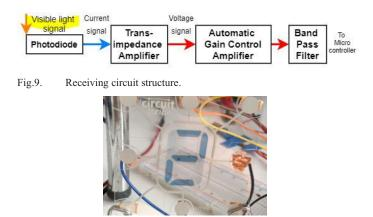
Fig.10. Electrochromic seven segment display developed by Ynvisible.
