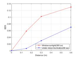
Fig.13. BER vs distance under different environment.
