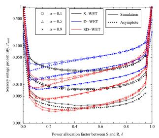
Fig. 2. Secrecy outage probability vs. power allocation factor  $\delta$  in the IT phase, for  $\alpha = 0.1, 0.5, 0.9$ , with  $\mu = 0.5$  and  $\gamma_P = 30$  dB.
