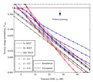
Fig. 1. Secrecy outage probability vs. transmit system SNR, for  $\delta=0.1,0.5,0.9,$  with  $\alpha=0.5$  and  $\mu=0.5.$
