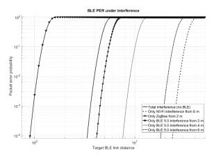
Figure 7. PER results for link on-body BLE to off-body BLE.
