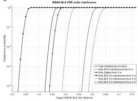
Figure 6. PER results for a WBAN on-body BLE link.
