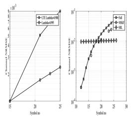
**FIGURE 6.** Channel NRMSE versus symbol no, (a) Practical 3 G LTE channel,  $\lambda = 0.988$ ,  $\lambda = 0.995$  and (b) Comparison of MSKF with SBL, J = 50, K =1, SNR = 10 dB, 14 iterations/stages.
