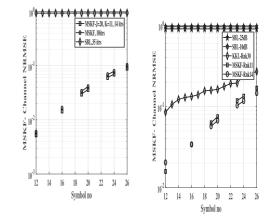
**FIGURE 7.** (a) Large scale systems, channel NRMSE versus symbol no, J = 20, K = 11, SNR = 10 dB and (b) J = 28, K = 14, MSKF with < 14 iterations, SNR = 10 dB; SBL: 100 iterations, SNR = 10 and 35dB.
