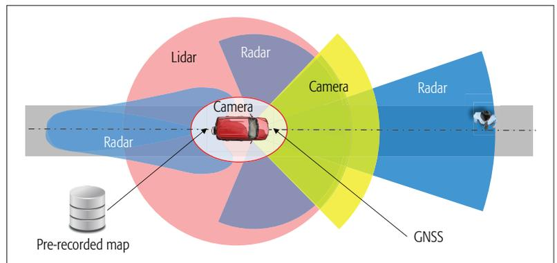
**FIGURE 1.** Main positioning technologies for automotive applications. In addition to signals from GNSS satellites, a variety of relative positioning technologies (with indications of their relative range) are available. These can be combined with a pre-recorded map to provide accurate absolute positioning.
