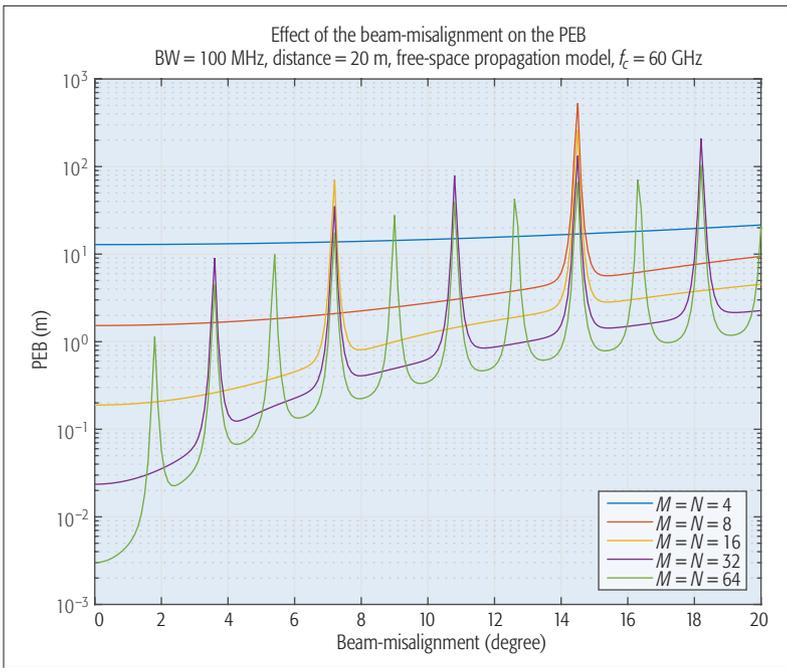
**FIGURE 2.** Positioning performance (PEB, indicating the positioning accuracy that can be achieved) of a vehicle for different numbers of transmit antennas  $N$  and receive antennas  $M$ , using a 100 MHz signal centered around a 60 GHz carrier from a single reference station. The figure shows that with more antennas, positioning accuracy improves, but becomes more sensitive to beam misalignment, which here is modeled by the receiver moving outside of the directions of the beams.
