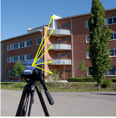
Figure 5. Yellow lines show direction of receiving antenna at the reference measurement.
