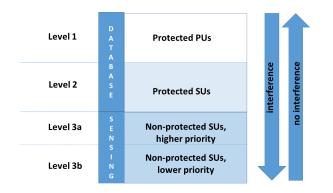
Fig. 3. Proposed spectrum sharing model.
