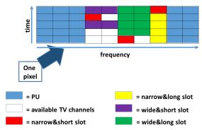
Fig. 5. Time and frequency resource allocation in one geographical pixel. Available channels can be narrow in frequency and short in time, narrow in frequency and long in time, wide in frequency and short in time, and wide in frequency and long in time.
