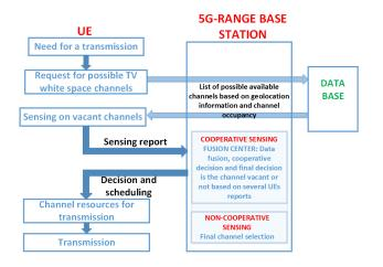
Fig. 7. Combining geolocation database and sensing information.
