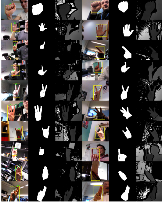
Fig. 1. Samples from the OUHANDS train (the image set on the left) and test (the image set on the right) databases. All the ten different hand poses are shown performed by different subjects. The first column shows the RGB data that has the bounding box and orientation normalisation information superimposed, the binary hand segmentation mask is in the middle column and the depth data is in the right column. Note that there is no orientation normalisation in the test set.
