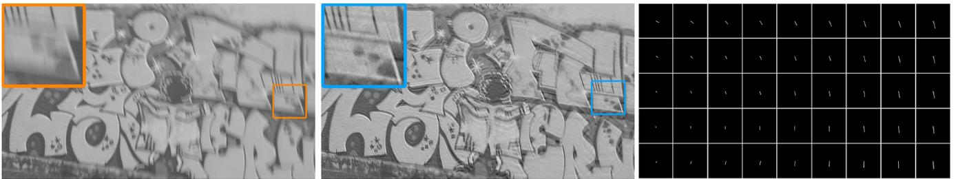
Fig. 3. A real-world image with spatially-variant motion blur (left). Deblurred image (center). Blur kernels calculated from IMU motion estimates (right).
